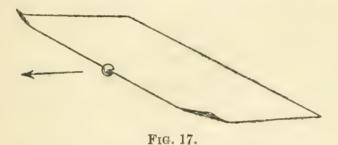
front edge, and the plane launched. The weight of the shot prevents the fore-edge from being tipped up; the apparatus therefore remains level, but pursues a regular downward path to the ground.<sup>2</sup> Some trials will be necessary before the exact weight which will give it its longest flight is discovered (Fig. 17).
